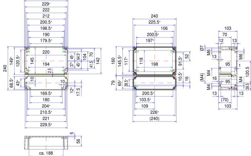
\* Please note: Mould slope for casting ejection, dimensions in the amount of the bottom!
