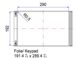
\* Please note: Mould slope for casting ejection, dimensions in the amount of the bottom!
