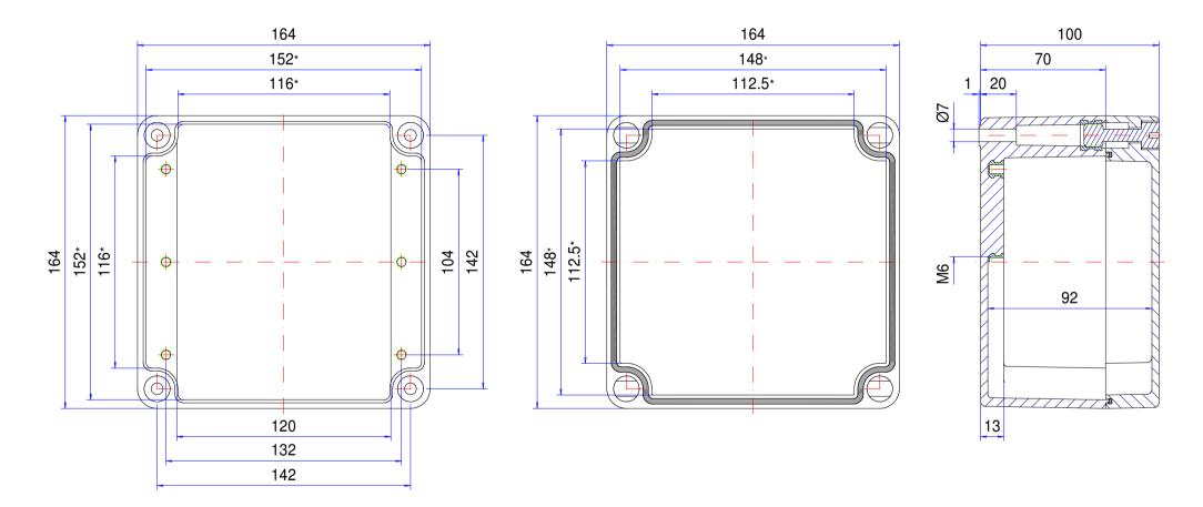
\* Please note: Mould slope for casting ejection, dimensions in the amount of the bottom!
