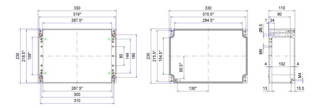
\* Please note: Mould slope for casting ejection, dimensions in the amount of the bottom!
