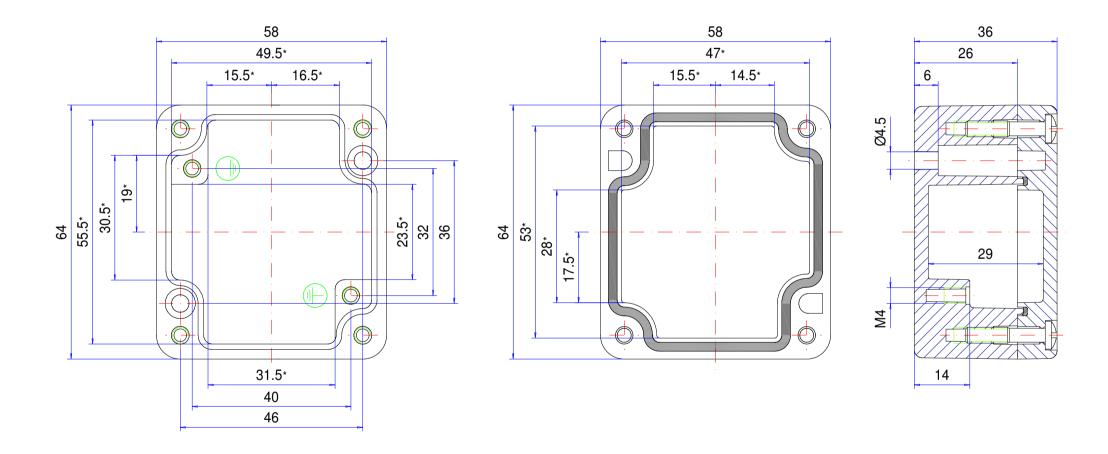
\* Please note: Mould slope for casting ejection, dimensions in the amount of the bottom!
