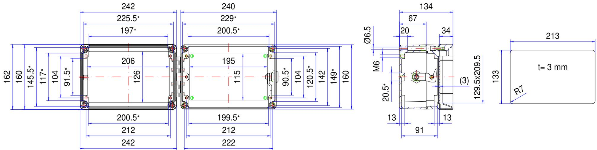
\* Please note: Mould slope for casting ejection, dimensions in the amount of the bottom!
