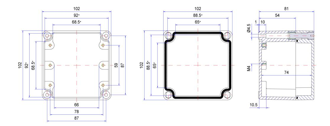
\* Please note: Mould slope for casting ejection, dimensions in the amount of the bottom!
